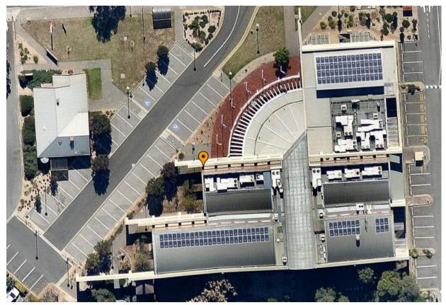
Figure 6: option for 32.5kW of solar PV on the admin building
