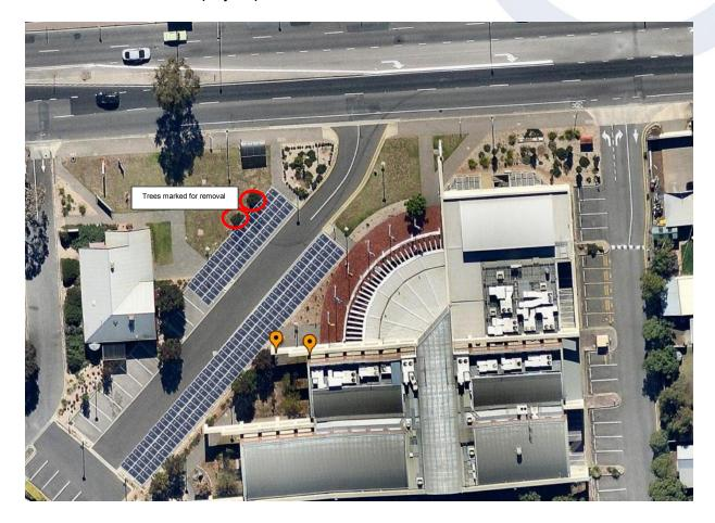
Figure 8: Proposed 55kW Carport Solar array
