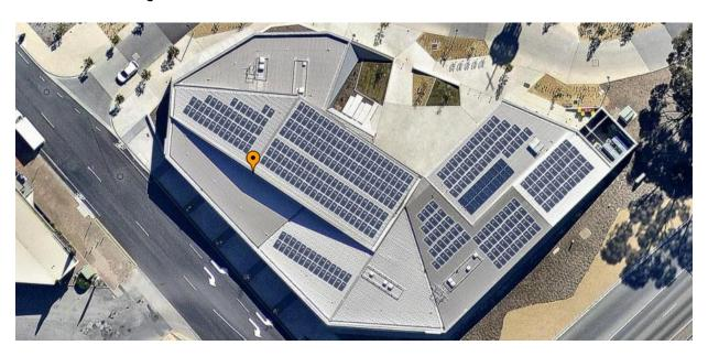
Figure 3: Potential layout of 100kW of Solar PV array
