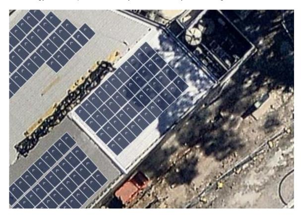
Figure 4: Shade affected North-East facing array (11kW)
