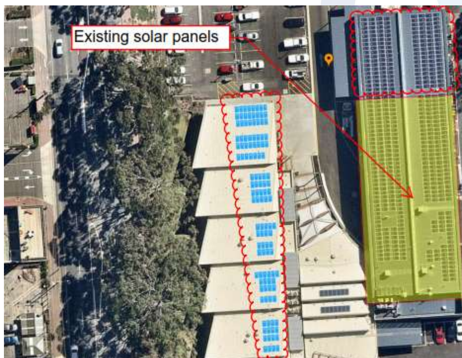
Figure 2 - Indicative layouts for additional solar panels on the City Services depot roof areas
