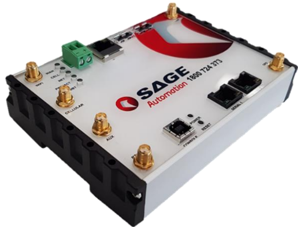
Figure 3- SAGE Edge pedestrian detection device
