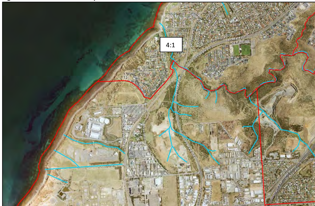
Figure 18: Stormwater flow paths in Field River area
