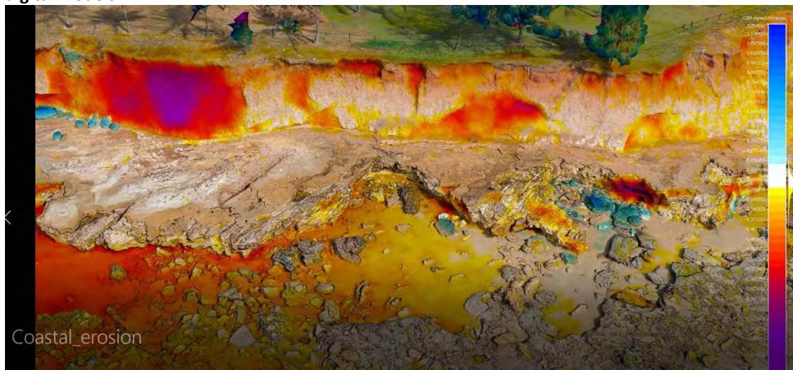
Figure 27: Changes to coastal environments can be accurately assessed and graphically portrayed with 3D digital models
