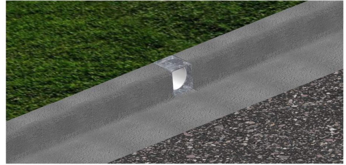
KERB INSERT ADJACENT TO GRASSED (UNPAVED) VERGE
