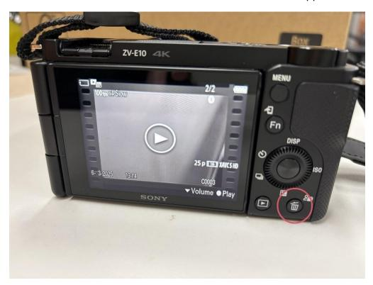
4. Use the outer button to highlight delete. Select delete by pressing on the central button.
